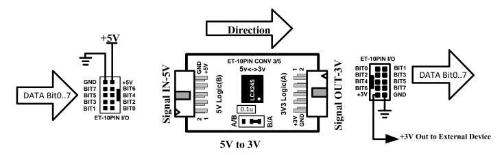
2.) Convert Logic from 3V to 5V: It has to set Jumper to the position of A/B; Port on the side of Logic (B) interfaces with +5V(PIN9) and GND(PIN10); and PIN1-8 is Signal Output Level 5V that has been sent from the side of Logic (A) to drive LOAD 5V or interface with Pin INPUT of MCU 5V. On the side of Logic (A), Pin 1-8 is used to receive external Signal that is Logic level 3V-3.3V to convert into Level 5V.
